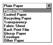
The Print Media <u>Combobox</u> is used to define the type of print media (such as plain paper, or Transparency film) that is loaded in the Canon Bubble Jet printer. This setting is important for controlling the quality of the final printed image. Specifying the correct Print Media setting is essential for producing high-quality printed images.
